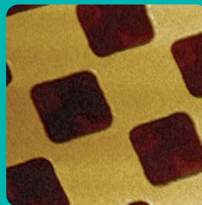
STM Image of 6µm pitch calibration grating at 300K
